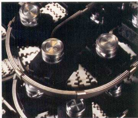
Alpine buffer Alpine pallet buffering (in-/off-line) and elevation of pistons on pallets.
