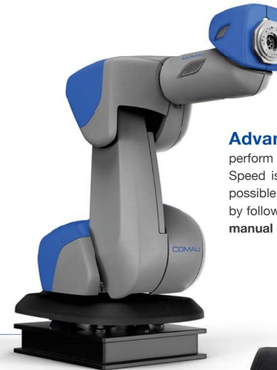
**Advanced Use Robotic Arm:** AURA supports humans perform manual operations by optimizing the work process. Speed is tuned, depending on the device's signals which makes it possible for the robot to move in free space or in contact operations by following programmed trajectories or learning from the operator in manual guidance.
