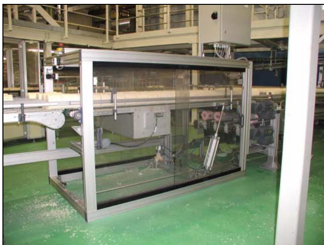
Pneumatically driven vertical diverter with four lanes, one in-feed level and two discharge levels.
