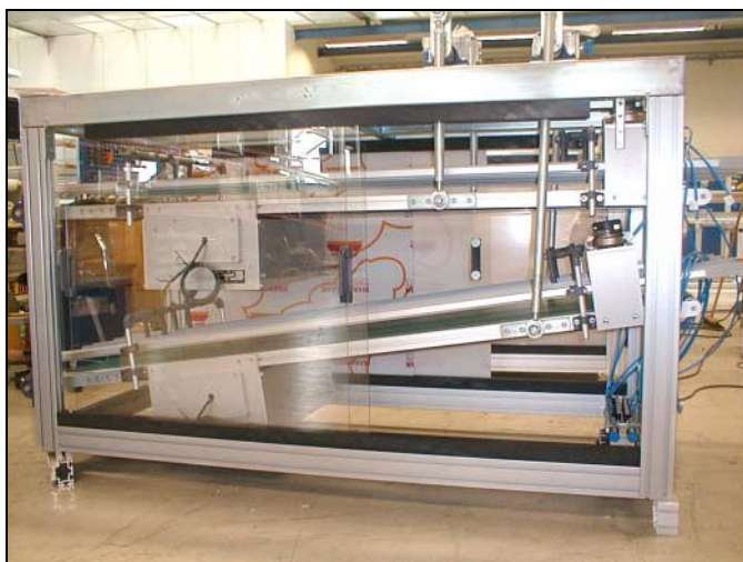
Three-lane diverter driven by electrical motor and crank, with two in-feed levels and three discharge levels.
