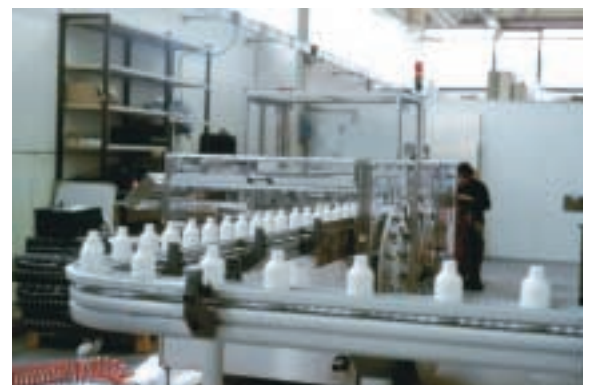
Pharmaceutical bottles exiting blowing machine
