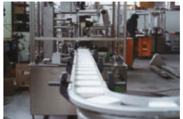
In-feed of labeller for pharmaceutical products
