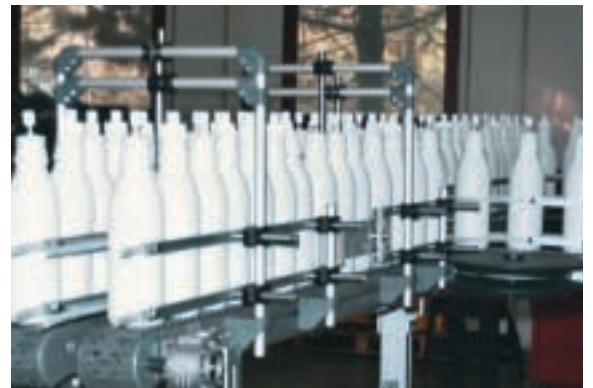
Parallel EM conveyor tracks transporting plastic bottles
