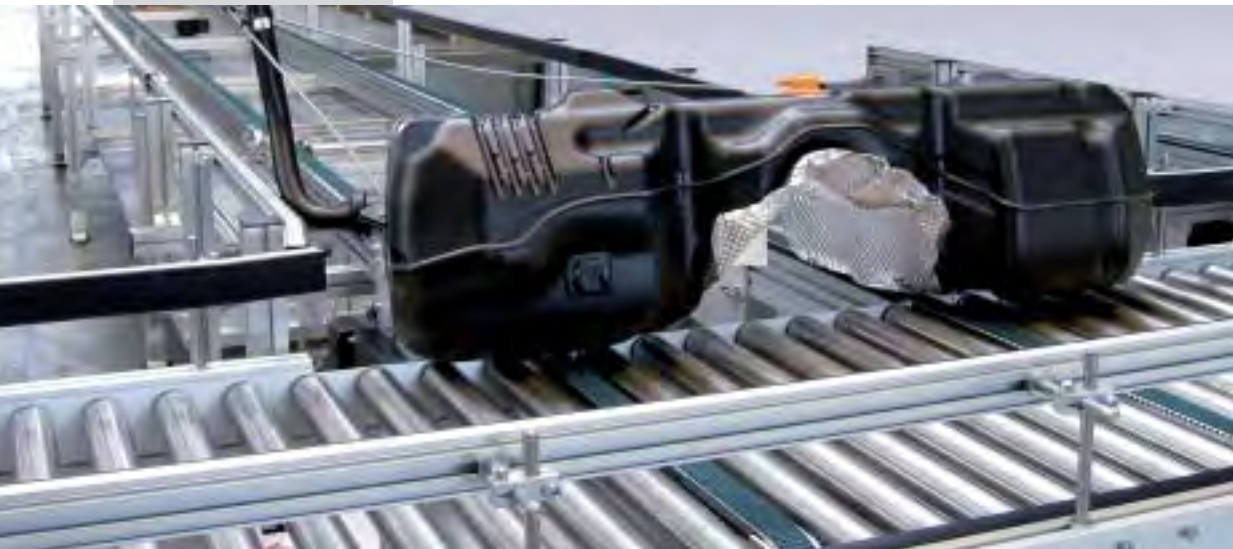
RBT-P 2255 with integrated lift and transfer conveyor, belt loading capacity 100 kg/m with additional side rails and drip pan
