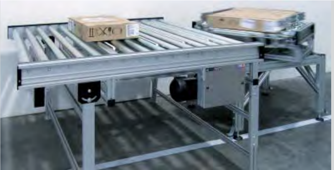
Combination of turn table and RBT-P 2255 with buffer table for order picking tasks and \varnothing 50 mm steel rollers. Driven via tangential chain drive
