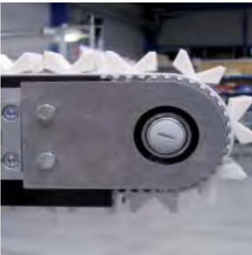
Tail ZRF-P 2040.02 with prismatic cleats
